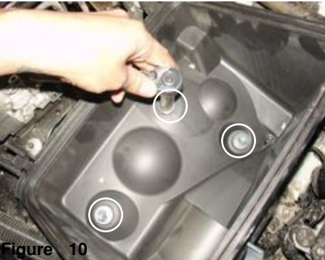
Figure 7 With 10mm socket and ratchet, loosen the 3 screws holding in the upper part of the factory air box.
