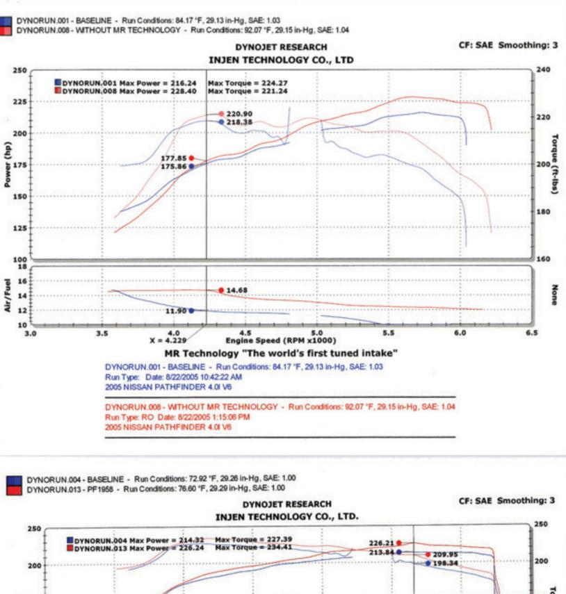
MRtech1 This graph without the use of MR Technology, reveals a very unstable and lean air/fuel ratio while making high horsepower/torque gains.
