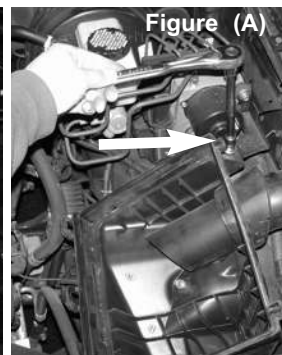
Remove 10mm bolt located on the right upper portion of the air box (Figure A). Lift air box up and off the lower grommet located at the bottom of the air box. Stock air box component removal is now complete.
