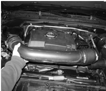
With both clamps loosened, remove entire air duct with the air resonator box attached.
