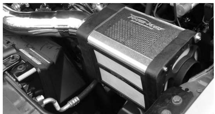
Here is a side view of the Power box installed and connected to the vibra-mount stud and air intake inlet.
