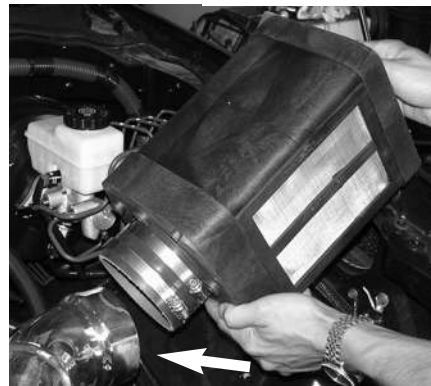
Postion Power-flow box in the engine compartment and press four inch hose over the intake inlet as shown in this picture .
