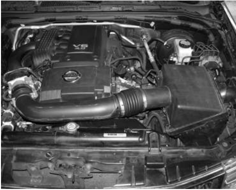
Picture of factory air intake system
