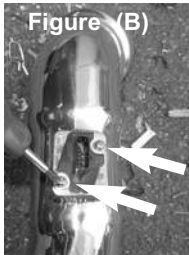
Place the MAF sensor onto the sensor pad on the Injen intake pipe. (Figure A) Re-use the two MAF screws to mount the MAF sensor on the sensor pad. (Figure B) Re-connect the MAF sensor harness, make sure you press firmly.
