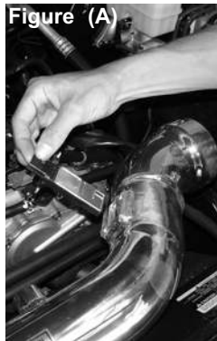
Place the MAF sensor onto the sensor pad on the Injen intake pipe. (Figure A) Re-use the two MAF screws to mount the MAF sensor on the sensor pad. (Figure B) Re-connect the MAF sensor harness, make sure you press firmly.
