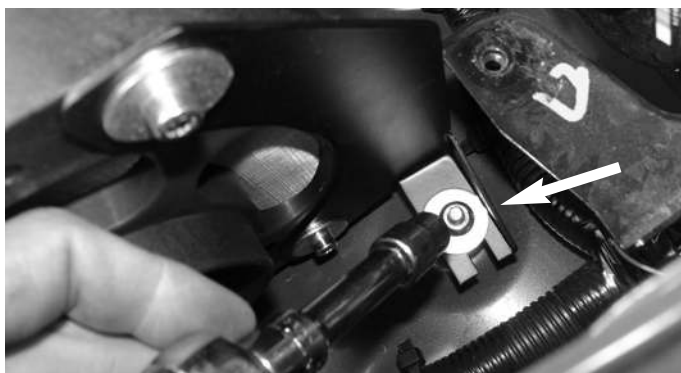
Align the Power box mounting bracket to the vibra-mount stud and use the m6 nut and fender washer to secure the box in place.
