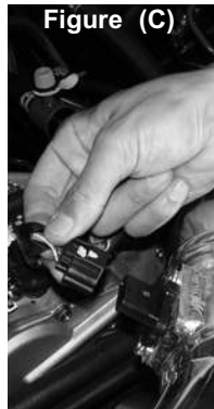
Place the MAF sensor onto the sensor pad on the Injen intake pipe. (Figure A) Re-use the two MAF screws to mount the MAF sensor on the sensor pad. (Figure B) Re-connect the MAF sensor harness, make sure you press firmly.
