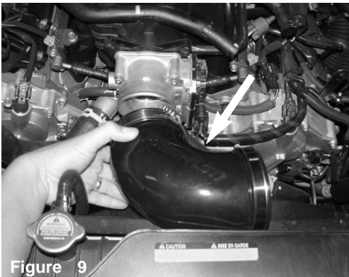
Figure 6 Unplug the MAF sensor harness from the MAF sensor
