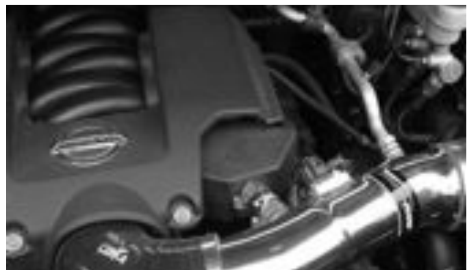
The plastic intake manifold cover is placed back to its original location. The CCV box will fit snug under the cover.
