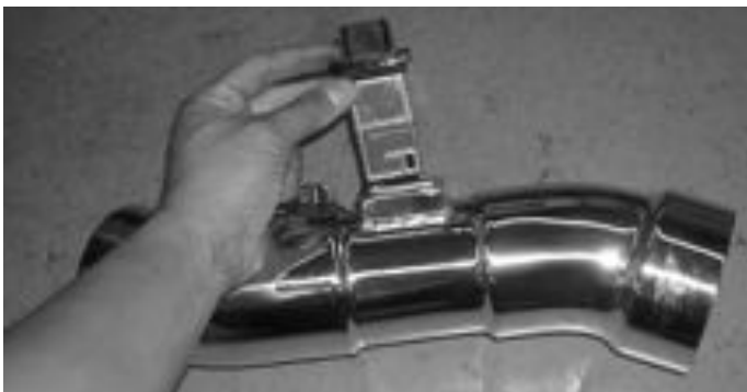
Insert the mass air sensor into the machined flange welded on the intake. Once the sensor has been firmly pressed into the flange, use stock screws to secure the sensor in place.
