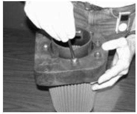
Unbolt the four- 12mm screws from the velocity stack base located to the center of the base. Now separate the base from the velocity stack.
