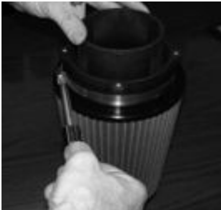
Loosen the clamp on the filter neck in order to separate the filter and velocity stack.
