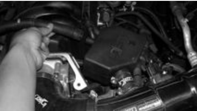
Locate the passenger side breather hose and press it over the CCV box port as shown in this picture.
