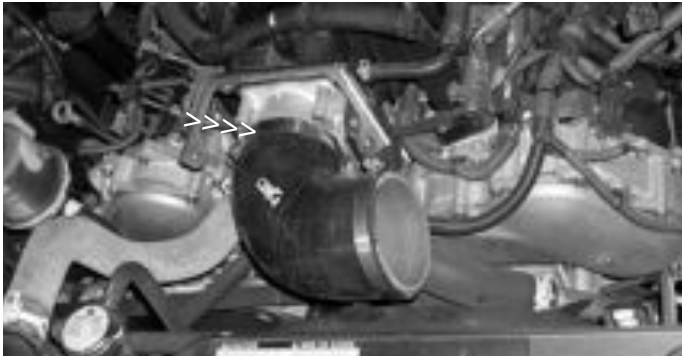
Place one large (.056) clamp over the end on 90 degree silicone elbow then press the 3 1/4" end over the throttle body. Semi-tighten the clamp located on the throttle body side.
