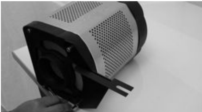
The bracket holes are lined up to the bolt pattern and the two 45mm screws are replaced. The bracket is now secured to the Power box.
