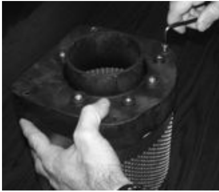
Unbolt the four- 65mm screws from the velocity stack base located on the corners of the base.
