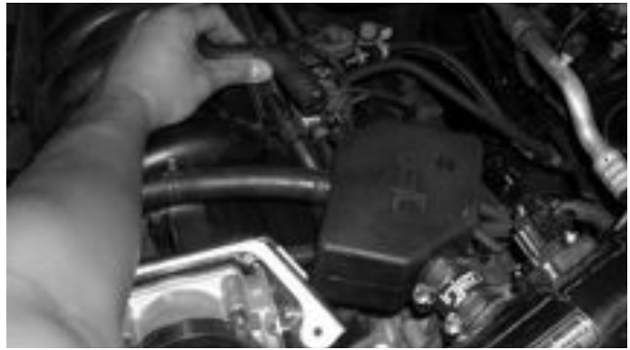
Locate the driver side breather hose and press it over the CCV box port as shown in this picture.
