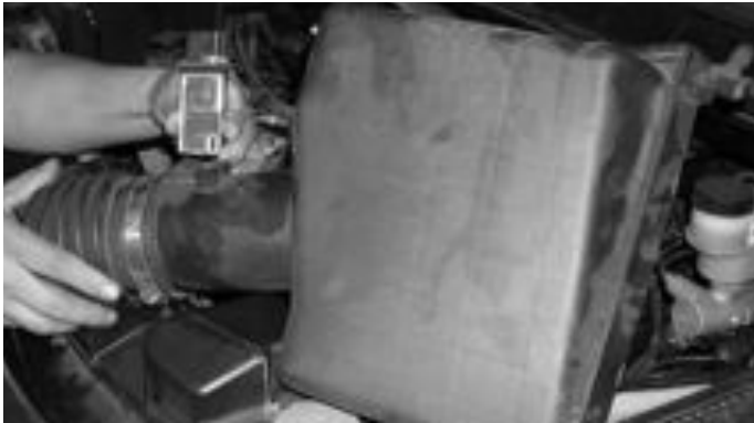
Remove screws holding the sensor in place and carefully slide the mass air sensor out of the sensor pad located on the air box outlet.
