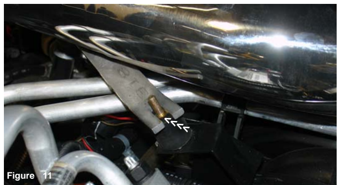
Figure 8 Align and screw the vibra-mount into the pre-tapped metal clip on the intake manifold.
