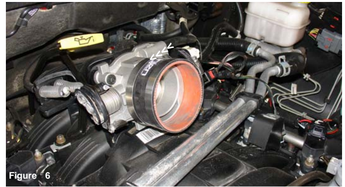
Figure 4 The arrow indicate where the sensor has been removed and placed to one side. Now, the first intake plenum mounting bolt is removed, the bolt is located on the driver side as indicated by the circle.
