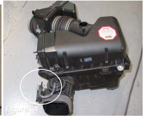
Figure 4 Note, the vacuum switching valve is intact with the air intake box which is no longer used.
