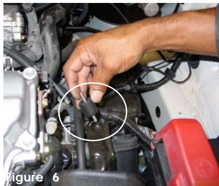
Figure 6 Take the 6mm vibra-mount and screw it into the stock air box bracket. Make sure it is fully screwed into the pre-tapped hole.
