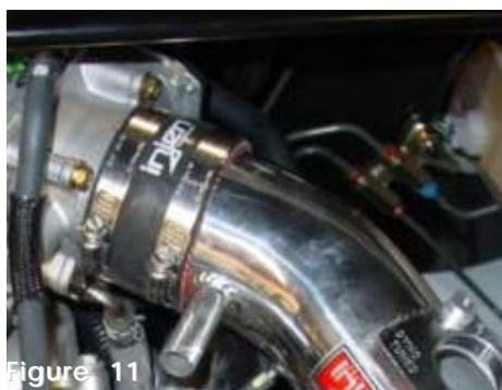
Figure 11 Once the intake has been adjusted continue to semi-tighten the clamp on the hose.
