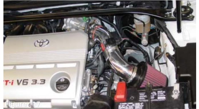
Figure 17 Top view of the air intake fully installed. Be sure to tighten all nuts, bolts, and clamps once the intake has been carefully aligned. Check the intake and vacuum lines for any rattling and/or vacuum leaks before moving forward with the test drive.
