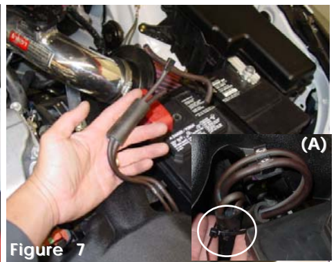
Figure 7 Take the wires that were connected to the vacuum switching valve and wire tie them away in a safe place. (See fig. A) The flapper valve has been illuminated so these wires can be tucked away in a safe place.
