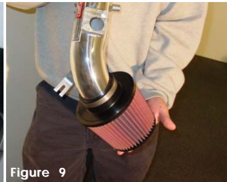
Figure 9 Press the filter on the end of the intake and tighten the clamp on the filter neck.
