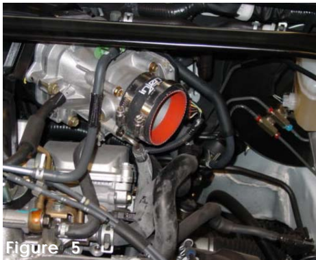
Figure 5 Place the 2 3/4" straight hose over the throttle body and use two clamps. Tighten the clamp on the throttle body side at this point.
