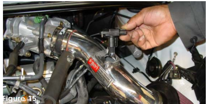
Figure 15 Remove the stock mass air flow sensor from the air intake box and press it into the machined adapter on the intake. Be sure not to break or pinch the O-ring along the base of the mass air flow sensor.
