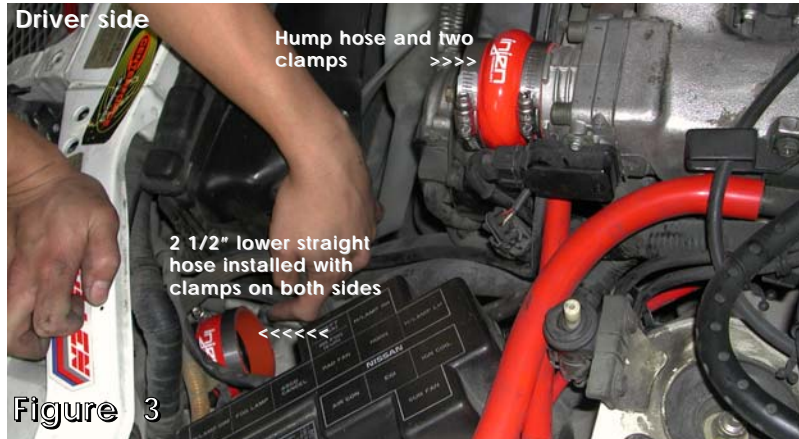
The 2 1/2" straight hose and hump hose have replaced the stock air intake ducts.
