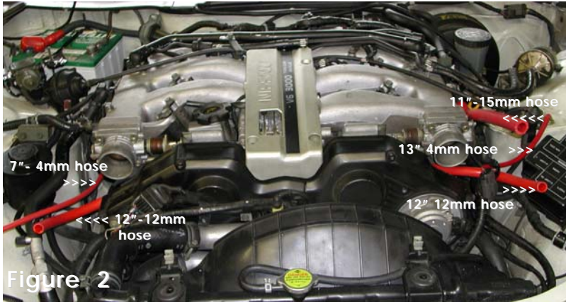
Front view of the engine compartment with stock air lines and air ducts removed. The stock lines have been replaced with the new Injen vacuum lines.
