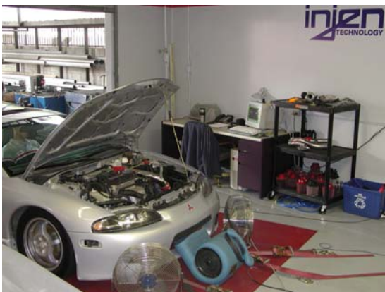
Injen Research and Development Team testing various proto-types on the dyno-jet. Both short intakes and cold air intakes are tested repeatedly.
