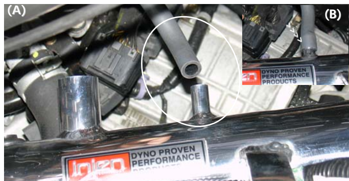
Insert the stock 8mm hose over the 3/8" intake port (A). Press the breather line just enough to hold itself in place (B).
