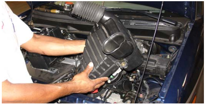
Note: For this installation, it will be required to remove the front bumper. Once the bumper has been removed continue to remove the stock air intake resonator from the bumper area.
