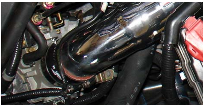
Press the intake throttle body side into the 2 3/4" hose. Align the intake bracket to the vibra-mount stud. Once the bracket has been aligned continue to semi-tighten the clamp on the intake.
