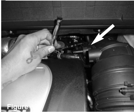
Figure 7 Use a 10mm socket and ratchet and loosen the 10mm clamp bolt on the air duct located on the Turbo charger compressure outlet. Pull the air duct from the outlet.
