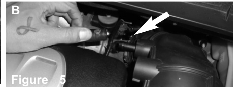
Figure 5 Figure A: Disconnect the recirculating diverter valve hose from the intake duct. Figure B: Disconnect the crank case breather line from the air duct.
