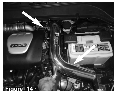
Figure 14 Position the intake pipe into the engine bay and place the end of the pipe into the steop hose on the turbo compressor outlet.
