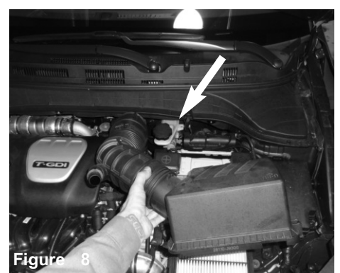
Figure 8 Remove the entire upper air box assembly and air duct from the engine bay
