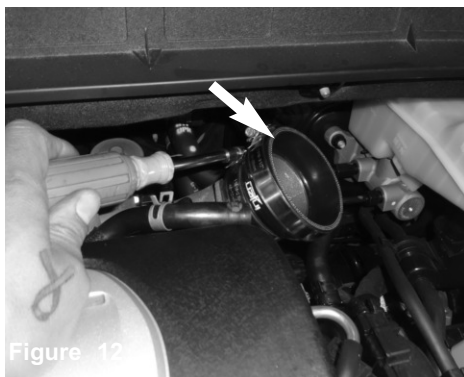
Figure 12 Place the 2.5"x3.00" step hose, #40 and #48 clamp onto the turbocharger compressor outlet.
