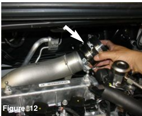
Figure 12 Place the 2.75\"X3.00\" step hose, #40 and #48 clamp onto the turbocharger compressor outlet.
