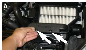
Figure 7 Use a 10mm socket and ratchet and loosen the 10mm clamp bolt on the air duct located on the Turbo charger compressor outlet. Pull the air duct from the outlet.
