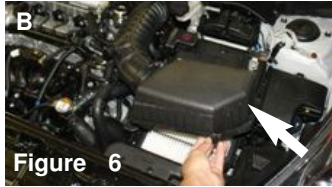
Figure 6 Figure A: Unclip the two tabs from the lower air box assembly to the upper air box assembly. Figure B: Detach the upper air box assembly from the lower assembly
