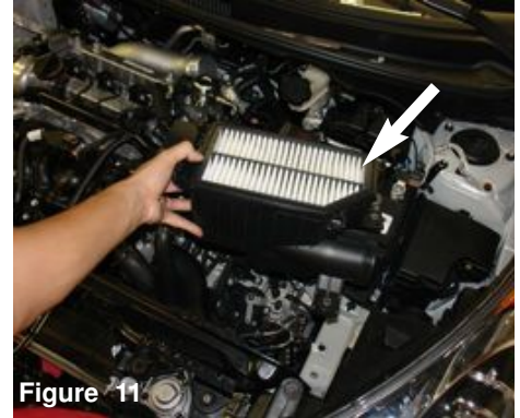
Figure 11 Now the lower air box assembly can be removed from the engine bay.
