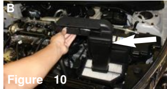
Figure 10 Figure A: Use a phillips screw driver and remove the two plastic screw clips from the front air intake duct Figure B: Lift up and remove the front air intake duct
