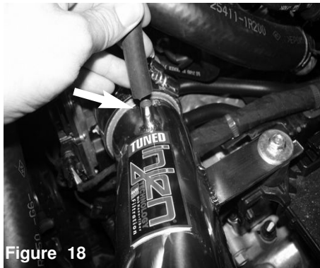
Figure 19 Install the air filter and tighten using 8mm nut driver.
