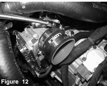
Figure 12 Install the step hose with clamps provided to the throttle body. Tighten the clamp on the throttle body using 8mm nut driver.
