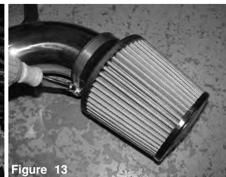
Figure 13 Install the air filter to the intake tube and tighten using 8mm nut driver.
