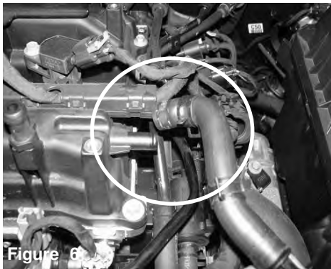
Figure 6 Remove the crank case line from the vehicle. If equipped with the brake booster line, disconnect from the intake and save for later install.
