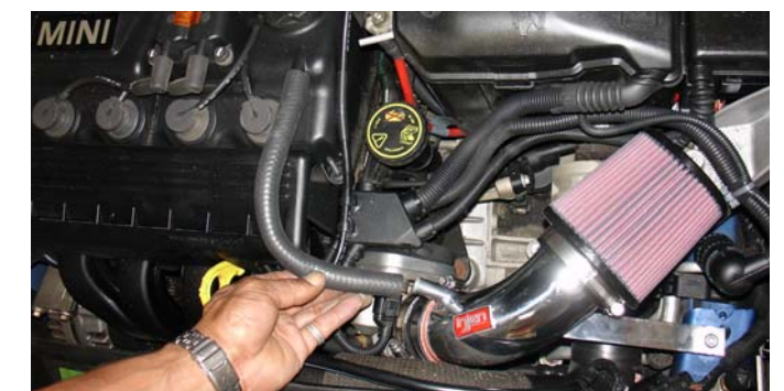
Once the intake has been align for best possible fitment, take the 12mm heat hose and press one end over the crankcase port.
