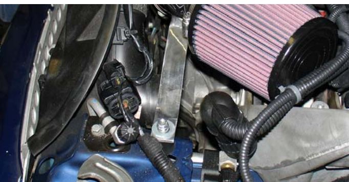
Take the flange nut and fender washer and secure the entire intake to the vibra-mount.
