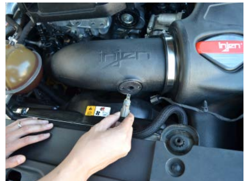
20. Install the IAT sensor into the air temp sensor adapter. Once full seated, twist the sensor to secure it.
