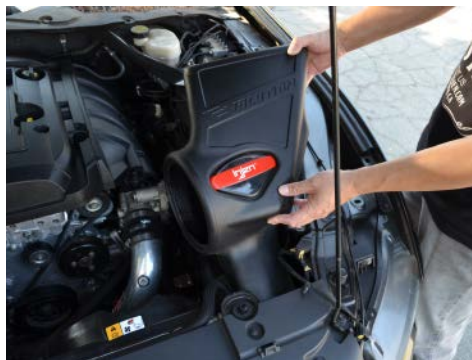
11. Install the injen air box into the engine bay.
