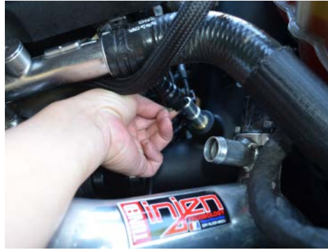
17. Connect the crank case line onto the machined fitting located on the injen tube
