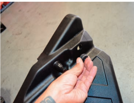
10. Install the smaller grommet and aluminum spacer from figure 8 into the injen air box.
