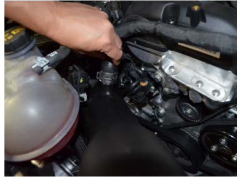
18. Connect the diverter valve return line to the injen intake tube. Then secure it using the OEM tension clamp.
