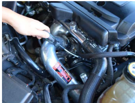
20. Insert the injen intake tube into the hump hose and secure the tube using the provided clamps.
