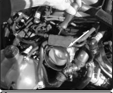
**6.** Install the urethane step hump hose to the throttle with clamps provided and tighten clamp on throttle body only.
