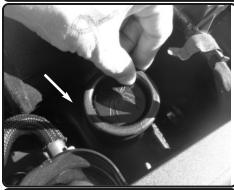
**5.** Install the provided filter monitor pluginto the slot. ( Sold seperately is our injen filter monitor see injen for more info)
