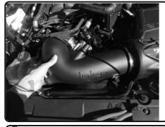
**7.** Place the Injen intake tube onto the throttle body and twist lock filter. Adjust the tube for best fitment and then secure the clamps.
