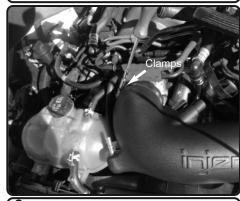
**8.** Adjust the tube for best fitment and then secure the clamps.
