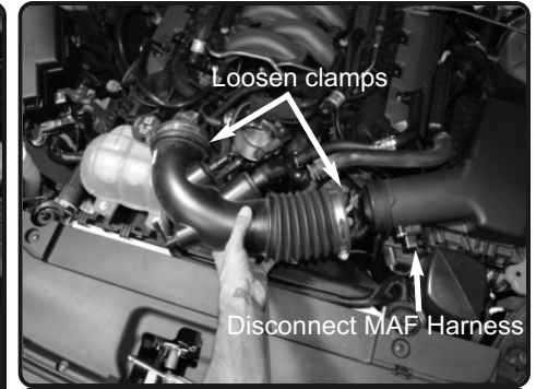
4. Loosen the two clamps on the factory air duct and then disconnect and remove from engine bay. Also disconnect the MAF sensor harness.
