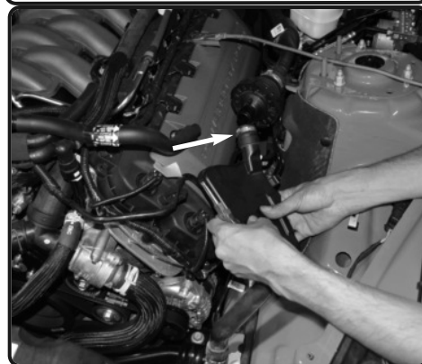
6. Disconnect the sound tube resonator box.
