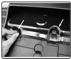
**15.** Re-use the two plastic retaining rivets from figure 2 to secure the Injen lower air box scoop to the radiator support
