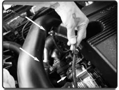
**23.** For the 3.5.L and Raptor models, pull back the Temp harness clips from the in-take tube, this will allow for more length to the sensor. Re-connect Temp harness.
