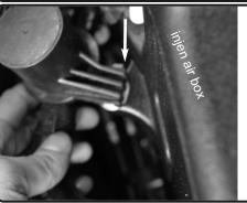
**19.** Attach the vacuum solenoid to the side of the air box.
