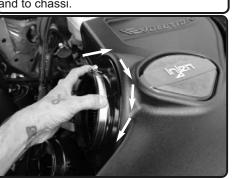
**16.** Install the twist lock filter into the injen air box.
