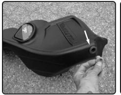
**12.** REmove the OEM grommet and crush washer from the stock airbox. Install into the new injen air box.
