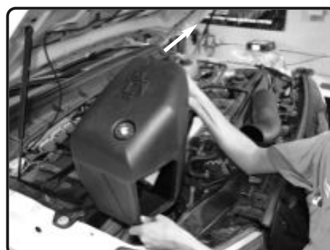
11. Drop the complete Injen airbox onto the mounting grommets from figure 10.
