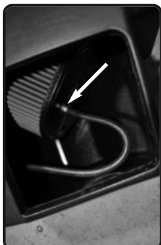
9. Connect the 3mm vacuum hose to the 1/8" fitting on the filter. Then connect the other end to the filterminder from figure 6.
