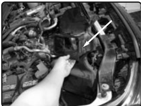
5. The plastic vent panel behind the passenger side headlight will have to be removed.
