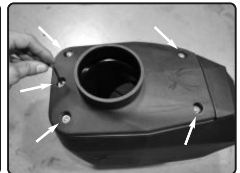
8. Place the five M8X12 bolts into the plenum and secure the plenum to the Injen airbox using an allen key.
