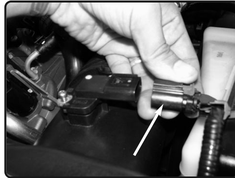
3. Disconnect the MAF sensor harness from the MAF sensor on the air box assembly.
