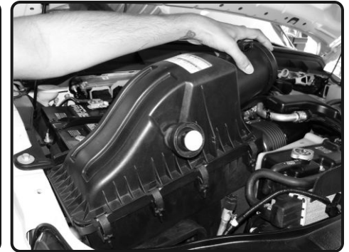
4. Lift the entire air box assembly out. Once air box is out. Remove the air duct from figure 3
