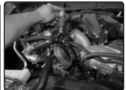
12. Place the 4.50" straight hose and two #72 clamps onto the turbo inlet. Only secure the clamp on the turbo inlet for now.
