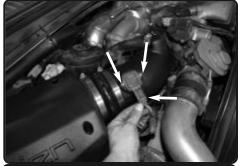
**20.** Use the supplied M4X10 bolts and secure the MAF sensor to the intake tube and then reconnect the MAF sensor harness
