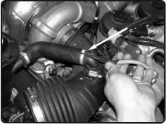
**2.** Use a needle nose plier and remove the permanent hose clamp on the factory air duct. A #16 clamp will be supplied to replace this clamp.
