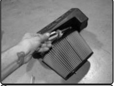
**8.** Place the filter onto the filter flange under the Injen air box plenum and then secure the clamp.
