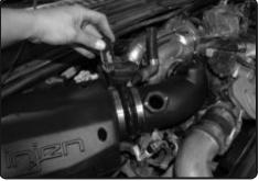
**18.** Once the Injen intake tube is in position, secure all the clamps
