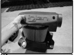
**10.** Place the Injen intake plenum onto the top of the Injen lower air box.
