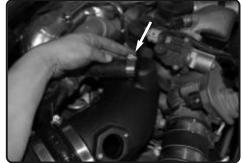
**19.** Use the supplied #16 clamp and secure the crank case vent tube to the port on top of the Injen intake tube.
