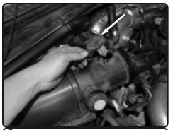
**5.** Unscrew the screws on the MAF sensor and then remove the MAF sensor from the factory air box assembly.
