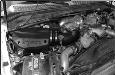
the installation of this intake system. Periodically, check the alignment of the intake, normal wear and tear can cause nuts and bolts to come loose. Note: Check clearance and adjust if needed! Failure to check the alignment and adjust the intake can cause damage that will void the warranty. Injen Technology is not responsible for any damages caused by/from improper installation.
