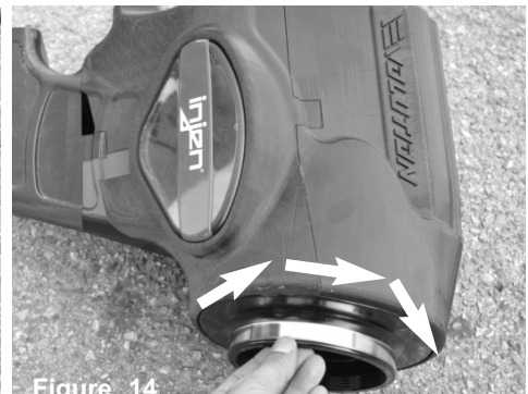
Figure 14 Once the filter is seated correctly, twist and turn in either direction a 1/4" turn.
