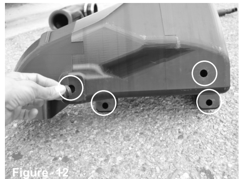
Figure 12 Remove the factory grommets from the OEM air box and install to the new injen air box.
