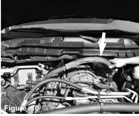
Figure 10 Remove the factory plastic hard crank case line out of vehicle.
