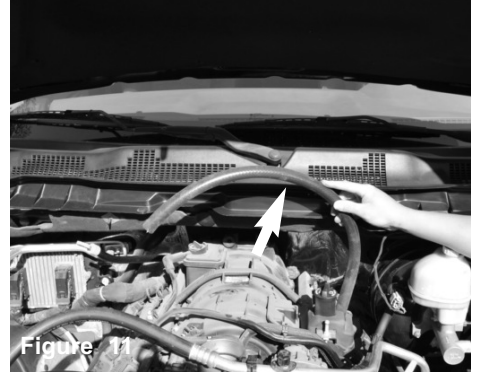
Figure 11 Install new provided 15mm crank case hose. Re install the engine cover.
