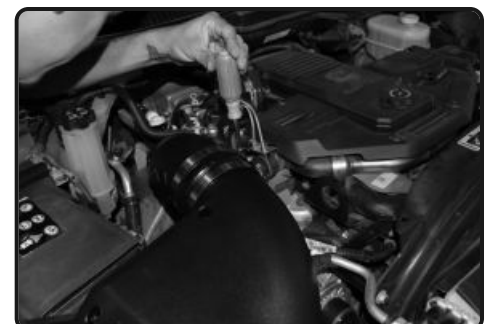
24. Slip the 4.50" hump hose over the air box plenum. Make sure it centered and the secure the clamps
