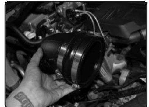
20. Place the 4.50" hump hose and two #72 clamps onto the top end of the intake tube.
