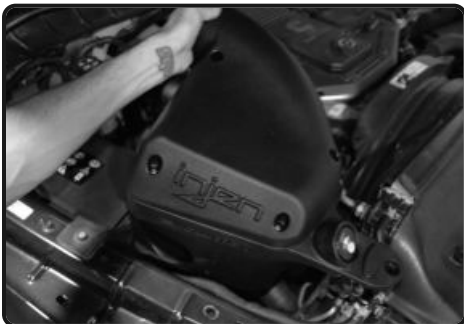
21. Lower the entire air box assembly into the engine bay. Make sure you line up the two mount tabs to the grommets on the chassis.
