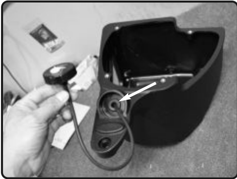
13. Install the grommet onto the air box bracket. connect the 3mm vacuum hose to the filter minder and then insert vacuum line and filter minder into the grommet.
