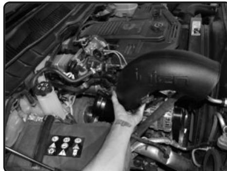
18. Attach the intake tube to the turbocharger and then connect the 15.9mm vacuum line to the CCV tube on the engine.
