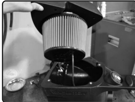
14. Connect the 3mm vacuum line from the filter minder to the fitting on top of the filter.
