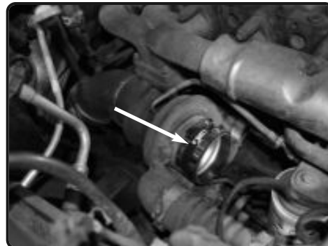
6. Place the 4.00" straight hose and two #72 clamps onto the turbocharger inlet
