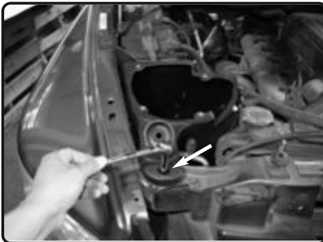
9. Once the Injen air box is mounted, use the factory 10mm bolt to secure the air box bracket to the radiator support.
