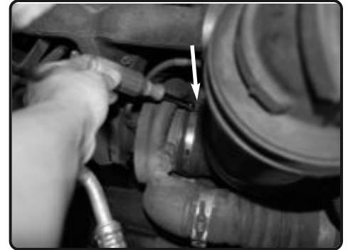
4. Loosen the clamp on the stock air box assembly air duct to the turbocharger
