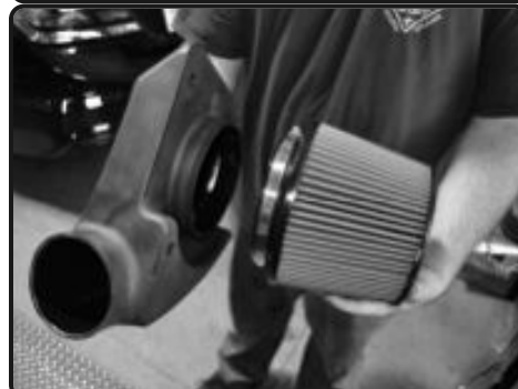
11. Place the filter onto the 6.00" opening on the intake plenum and then secure the clamp.
