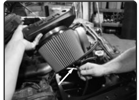
12. Connect the 3mm vacuum hose from figure 10 to the Filter Minder to the barbed fitting on top of the Injen filter.
