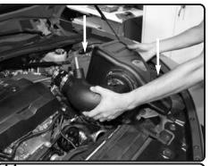
**14.** Now install the intake into the vehicle. Position the tabs on air box to OEM grommet locations. Position the tube to the turbo. *Do not tighten.*
