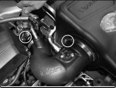
**16.** Adjust if needed, secure and tighten the clamp on turbo using 8mm nut driver. Tighten clamp on filter also.
