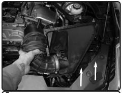
**5.** Now Lift up air box from vehicle and remove complete stock air box assembly.
