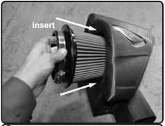
**8.** Install the filter into the passenger side air box housing. Position the Twist-Lock™ filter pattern to the hole cut out on air box.
