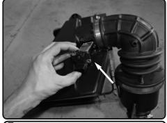
**7.** Remove the MAF sensor from the stock air box.
