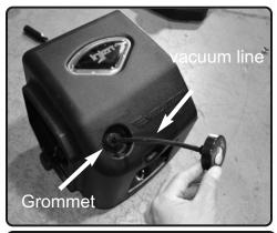
1. Connect the 3mm vacuum line to the Filter Monitor. Place the grommet into the 3/4" in the air box. Then run the 3mm vacuum line through the grommet.
