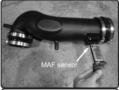
**18.** Install the MAF sensor into the intake tube and secure using provided M4 button head screws.
