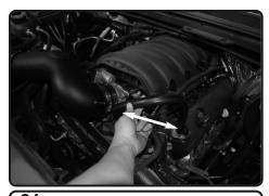
**24.** Install the provided 14.5" 15mm hose to the fitting on engine and intake tube on driver side.
