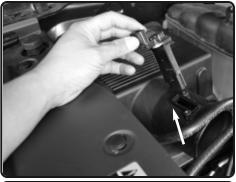
**4.** Pull the MAF sensor out of the factory air box assembly
