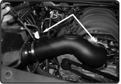
**22.** Install the intake tube. Secure the tube to airbox and throttle body. Position for best fit and tighten clamps. Re-connect the MAF sensor Harness.
