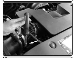
**5.** Loosen the clamp on the air box using 8mm nut driver.
