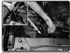
**19.** Loosen the support bar using 10mm socket or wrench. Push back for installation of air box.
