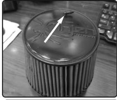
**2.** Drill a 0.1890" hole on top of the filter and firmly push the supplied 5/32 90 degree fitting into the hole.
