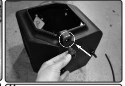
**11.** Now install the grommet spacer into the new injen air box and secure.
