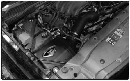
Congratulations! You have just completed the installation of this intake system. Periodically, check the alignment of the intake, normal wear and tear can cause nuts and bolts to come loose. <u>Note: Check clearance and adjust if needed! Failure to check the alignment and adjust the intake can cause damage that will void the warranty. Injen Technology is not responsible for any damages caused by/from improper installation.</u>
