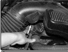
**6.** Unclip the coolant lines underneath the air duct from the tab
