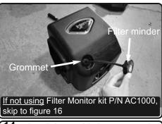
**14.** Install the provided grommet to the hole on air box, now attach the 3mm vacuum line to the filter minder and install the filter minder to the air box. Place hose through the grommet.
