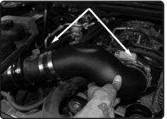
**23.** Install the intake tube. Position for best fit, secure and tighten all clamps using 8mm nut driver.
