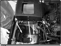
**19.** Now install the air box assembly into the vehicle. Position the tabs to seat like OEM box.
