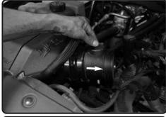
**22.** Install the MAF sensor to the hump hose. *Make sure Arrow on sensor is going in direction towards the throttle body.*
