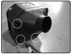
**17.** Now secure the plenum using provided 4 M6 screws and rubberized washers. Secure and tighten.
