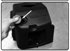
**12.** Push the Filter Monitor Plug into the Filter Monitor pod on the Injen air box if you are not using the Filter Monitor Kit P/N AC1000
