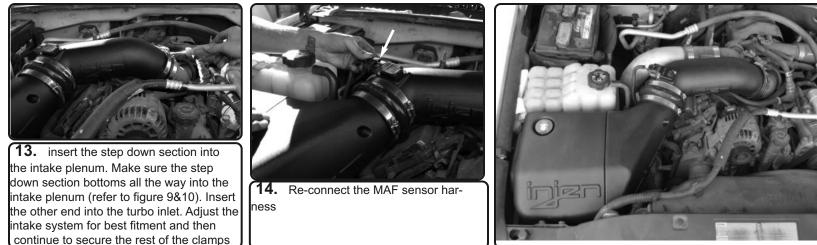
Congratulations! You have just completed the installation of this intake system. Periodically, check the alignment of the intake, normal wear and tear can cause nuts and bolts to come loose. <u>Note: Check clearance and adjust if needed! Failure to check</u> the alignment and adjust the intake can cause damage that will void the warranty. Injen Technology is not responsible for any damages caused by/from improper installation.
