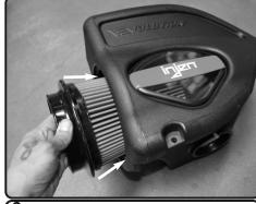
**8.** Insert twist lock filter to the air box.
