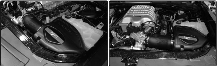
Congratulations! You have just completed the installation of this intake system. Periodically, check the alignment of the intake, normal wear and tear can cause nuts and bolts to come loose. <u>Note: Check clearance and adjust if needed! Failure to check the alignment and adjust the intake can cause damage that will void the warranty. Injen Technology is not responsible for any damages caused by/from improper installation.</u>
