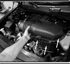
**6.** Carefully lift up and remove the stock air box assembly.
