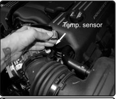
**2.** Disconnect the Temperature sensor harness.
