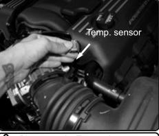
**2.** Disconnect the Temperature sensor harness.
