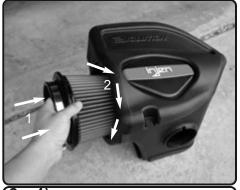
**8.** 1)Insert twist lock filter to the air box. 2)Once seated, rotate in either direction 1/4 turn till filter locks.
