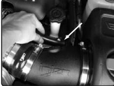
**15.** Place the Injen plenum onto the Injen lower air box assembly and use 4-M6X30 bolts to secure the plenum to the lower air box.
