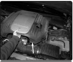
**2.** Lift up and remove engine cover.
