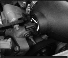
**19.** Once seated, rotate the sensor and secure.
