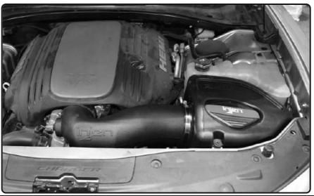
Congratulations! You have just completed the installation of this intake system. Periodically, check the alignment of the intake, normal wear and tear can cause nuts and bolts to come loose. Note: Check clearance and adjust if needed! Failure to check the alignment and adjust the intake can cause damage that will void the warranty. Injen Technology is not responsible for any damages caused by/from improper installation.
