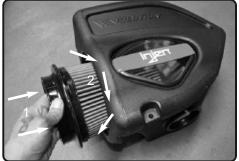
**10.** 1)Insert twist lock filter to the air box. 2)Once seated, rotate in either direction 1/4 turn till filter locks.
