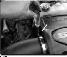
17. Secure the clamp on filter using 8mm nut driver.
