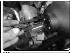
**18.** Install the Temperature sensor into the adaptor. Re-connect the Harness.
