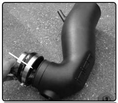
**12.** With provided Step hose and clamps install to the tube. Do not tighten.
