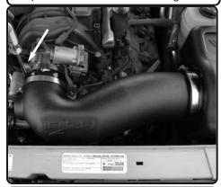
**16.** Secure the tube and position for best fit. Tighten clamp on Throttle body.
