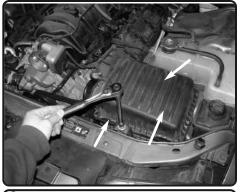
**8.** Use a 8mm socket with a 3/8 rachet and remove the 8mm bolt mounting the factory air box to the radiator support.
