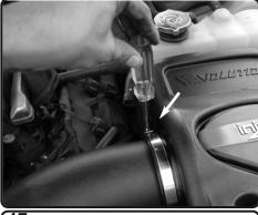
17. Secure the clamp on filter using 8mm nut driver.
