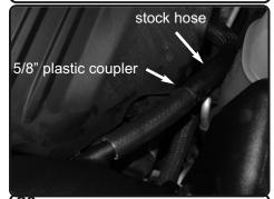
**20.** Install the provided 17mm hose and plastic coupler to the stock crank case hose. Connect the two and secure to the intake tube
