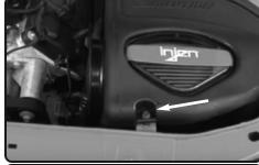
11. Install the air box assembly into the vehicle. Secure using OEM screw. Make sure the nipple fitting on back side of injen airbox is seated in the OEM grommet on fender well.
