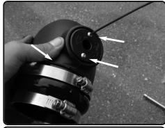
**14.** Secure the temp adaptor using the provided m4 button head screws. Tighten using 2.5mm allen key.
