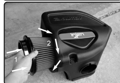
10. 1)Insert twist lock filter to the air box. 2)Once seated, rotate in either direction 1/4 turn till filter locks.
