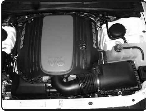
1. Stock air intake box and air intake duct shown above.
