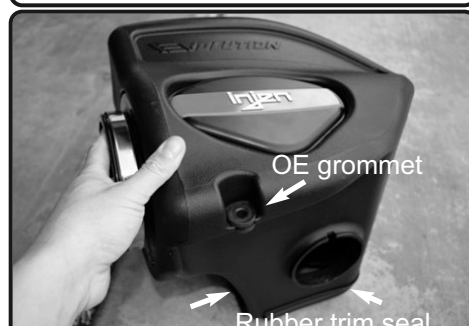
11. Remove the factory rubber grommet with washer from OEM airbox and install to the new injen airbox. Attach the Rubber trim to the bottom of the air box.
