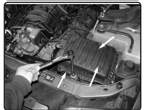
8. Use a 8mm socket with a 3/8 ratchet and remove the 8mm bolt mounting the factory air box to the radiator support.
