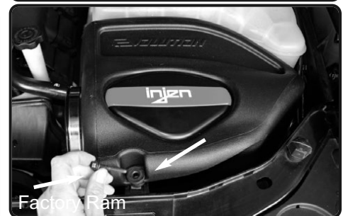
12. Install the air box assembly into the vehicle. Secure using OEM screw. Make sure the nipple fitting on back side of injen airbox is seated in the OEM grommet on fender well.
