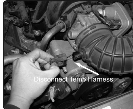
3. Once the engine cover is remove, disconnect the harness from the air temperature sensor.
