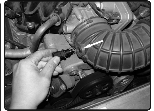
4. Firmly pull and remove air temperature sensor out of factory air duct.
