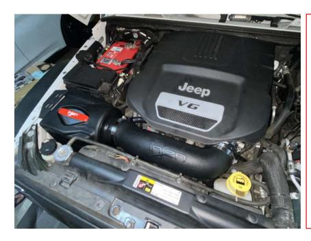
CONGRATULATIONS! You have just completed the installation of this intake system. Periodically, check the alignment of the intake, normal wear and tear can cause nuts and bolts to come loose. Note: Check clearance and adjust if needed!
