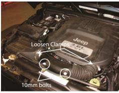
2. Remove the engine cover. Next loosen the two clamps from the intake tube. Finally, reomve the two 10mm bolts.
