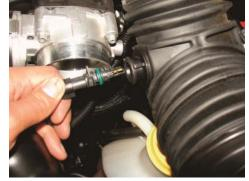
4. Twist the IAT sensor to remove the sensor from the intake tube.
