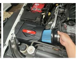
9. Install the twist lock filter on to the Injen air box. Once seated, rotate the filter a 1/4 turn in either direction so the filter can lock into place
