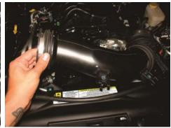
3. Disconnect the IAT harnes and remove the intake tube from the throttle body and air box.
