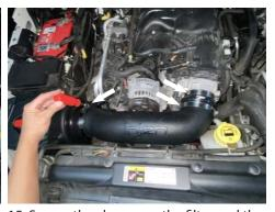
15. Secure the clamps on the filter and the hump hose.
