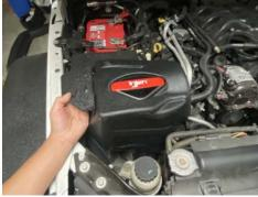
8. Install the Injen air box into the engine bay. Line up to the stock grommets and push down on the air box to secure.
