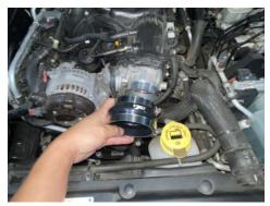
body and secure using the provided clamps.
