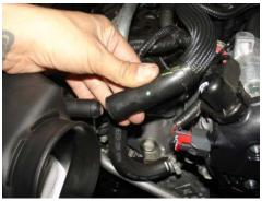
5. Disconnect the crank case breather tube from the stock air box.
