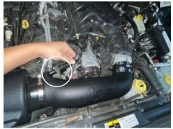
16. Reconnect the crank case breather hose to the injen tube.
