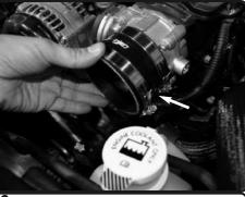
**6.** Place the 3.25"-3.50" step hose and one #48 and #56 clamp onto the throttle body.
