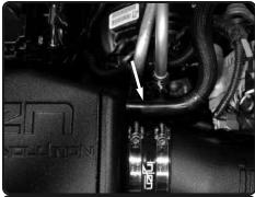
**15.** Connect the crank case vent tube to the port on the Injen air box assembly.
