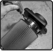
8. Place the filter onto the air box plenum and secure the filter to the plenum.
