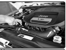
**14.** Insert the Injen intake tube into the hose on the throttle body and the hump hose on the Injen intake box assembly. Adjust the intake for best fitment and then secure all the clamps.
