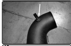
**12.** Place the grommet onto the 7/8" hole on the injen intake pipe and then insert the intake air temp sensor into the grommet
