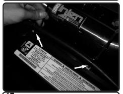
**17.** Zip tie the coolant overflow line from the coolant reservoir to the two threaded holes on the fan shroud.
