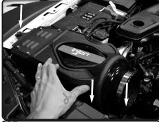
**15.** Install the airbox assembly into the vehicle. install into the factory position. Secure using the OEM screw from step 4.
