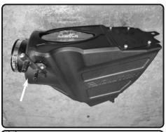
**14.** Air box assembly ready to be installed into the vehicle.
