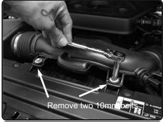
**3.** Loosen the 2 bolts holding in the intake tube and remove.
