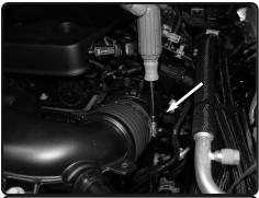
**5.** Loosen the clamp on the turbo inlet and pull back the intake tube from the turbo inlet.
