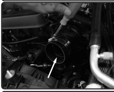
**8.** Install the provided step hump hose to the throttle body. Secure using provided clamps.
