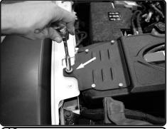
**18.** Once secured, tighten the bracket using 10mm socket or wrench.
