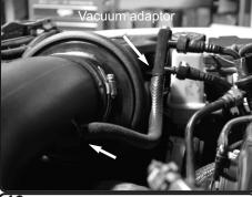
**19.** Connect the provided 10mm hose to the vacuum adaptor and to the brass barbed fitting on the intake tube. Adjust to desired position.
