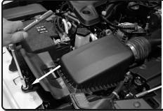
**4.** On the air box, loosen the bolt holding in the airbox. Loosen bolt and save for later install along with the grommet and crush washer.
