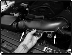
**6.** Lift up and remove the stock intake system out of the vehicle with air box..
