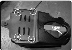
**10.** Secure the bracket to the air box using M6 socket cap screws. Secure and tighten using allen key.
