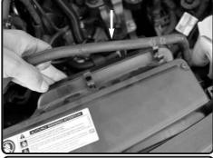
**7.** Loosen and pull back the coolant line from the OEM ram-scoop.
