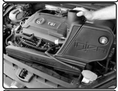
**5.** Install the intake assembly into the vehicle. Position to factory holes. Make sure the intake assembly seats in studs. <u>Note:Use</u> <u>lubrication to grommets for easier installation</u>.
