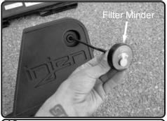
**12.** Attach the 3mm hose to the Filter minder and install the hose through the grommet.
