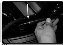
**12.** Connect the vacuum line and new hose together. This will have the extension to the brass 1/4" fitting on plenum.
