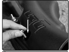
**3.** Install the plenum assembly into the air box. Secure using provided M6x20mm phillips screw with rubberized washer.
