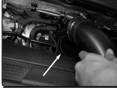
**4.** Pull back the intake tube from the turbo housing.
