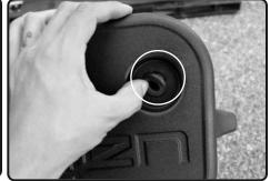
**11.** Install the provided grommet to the filter minder hole cut-out on injen air box.
