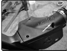
**4.** Tighten all the screws using a philips screwdriver.
