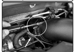
**9.** Position for the best fit. Tighten clamp using 8mm nut driver.
