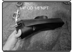
**9.** Install and secure the 1/8" NPT fitting to the plenum insert and tighten.
