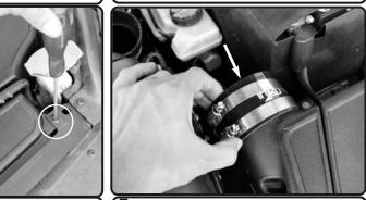
7. Install the 3.5" hump hose to the plenum. Do not Tighten.
