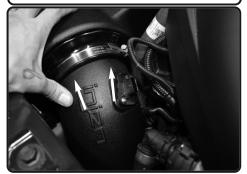
**23.** Once seated, install the intake tube into the filter.
