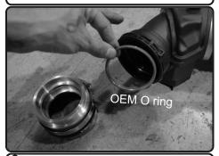
**9.** With a small flat head screwdriver, carefully pull out the OEM O ring seal.
