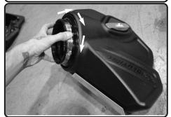
**21.** Once seated, turn the filter in either direction a 1/4" turn till the filter locks in place.
