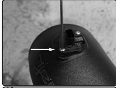
**16.** Re-install the temp sensor into the new injen intake tube and secure using the provided M4 button head screws.
