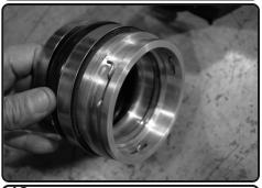
**12.** Turbo adaptor assembly. Make sure the OEM o ring and Lock clip are seated correctly.
