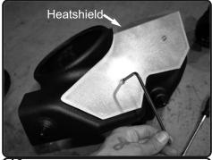
**19.** Install the heastshield to the bottom of the air box using provided M6 socket cap screws and tighten.
