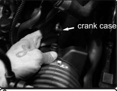
**6.** Disconnect the crank case line on the intake tube by depressing clip.
