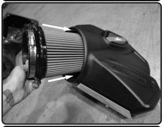
**20.** Install the twist lock filter to the inside of the air box.
