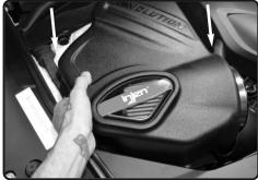
**22.** Install the air box assembly into the vehicle and position the studs to the grommets. Make sure the air box is seated.
