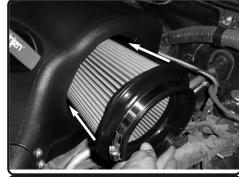
Insert twist lock filter to the air box.
