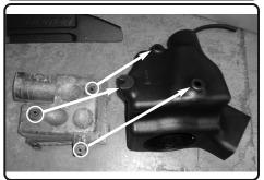
**11.** Remove the 3 grommet with crushwasher and install into the new air box.
