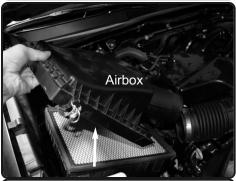
**4.** Un-clip upper half of airbox and remove from vehicle.
