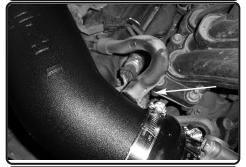
**22.** Re-connect the crank case line to the injen intake tube.
