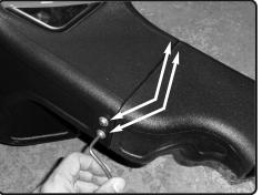
**14.** Secure the scoop to box using provided M6 button head screws and rubber washers. Secure and tighten using allen key.
