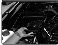
**7.** Now lift up and remove the lower part of the airbox out of vehicle.
