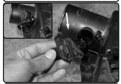
**8.** With phillips screwdriver, loosen the 2 screws holding in the MAF sensor. Carefully remove the MAF sensor.
