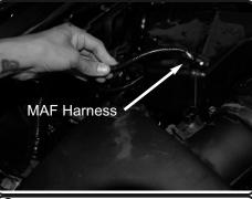
**2.** Disconnect the MAF sensor harness and pull line away harness from the airbox.
