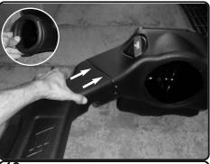
**13.** Install the rubber trim to the air box hole. Install the scoop to the air box.
