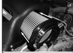
Insert twist lock filter to the air box.
