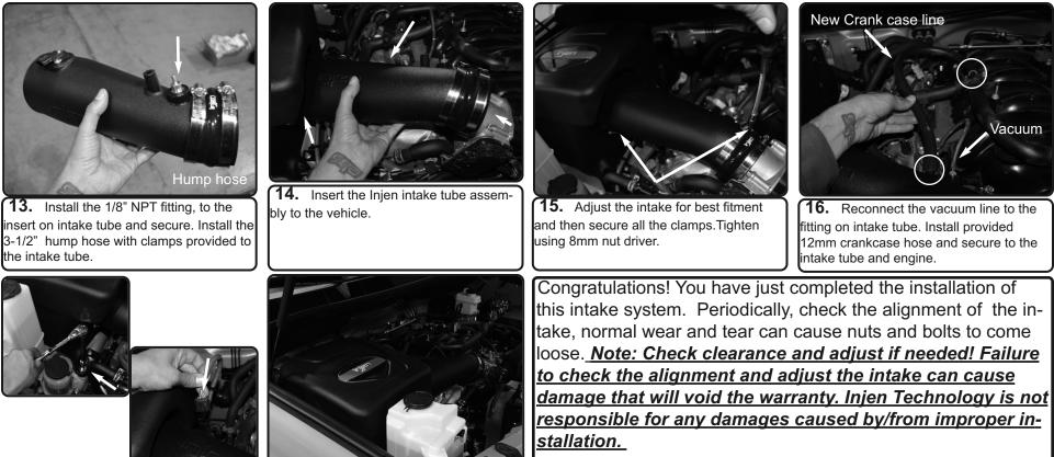
**17.** Secure the box and tighten using 10mm socket and wrench. Re-connect MAF sensor harness.
