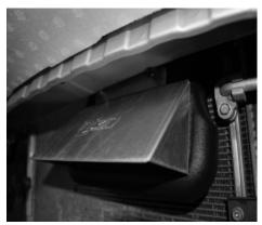
Rain guard installation is now complete. Re-install the the scoop assembly and secure the intake system. Note: Check clearance and adjust if needed! Failure to check the alignment and adjust the intake can cause damage that will void the warranty. Injen Technology is not responsible for any damages caused by/from improper installation.
