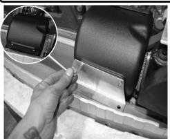
Remove front bumper cover. Loosen and remove the injen Evolution intake out of vehicle. Loosen the radiator support. (see injen Evolution instruction sheet EVO2000) Loosen the 2 socket cap screws from bracket and 2 plastic push clips. Push Injen ram scoop down allowing for access to inserts on scoop.
