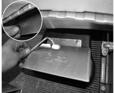
Install the rain guard. Secure using provided M6 socket cap screws and tighten. Once secure, cover the socket cap screw using provided vinyl cap. This will prevent any contact with screws and front bumper support. Failure to do so will result in vibration noise.
