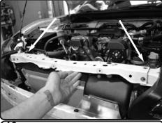
**19.** RE-install the radiator support and secure. Re-install the bolts and tighten.
