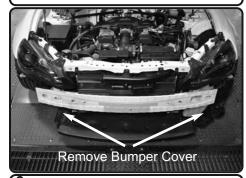
**9.** Carefully remove bumper cover. Remove the push-clips and 10mm screws on top and bottom and side and remove.
