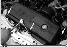
**35.** Secure and tighten all the screws using 10mm socket or wrench.
