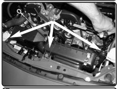
**7.** Loosen the 3 screws holding in the bottom half of the air box using 10mm socket and ratchet. Now lift up and remove the lower intake assembly from vehicle. Save for later install.
