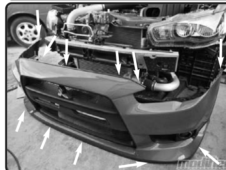
11. Removal of the front bumper will be necessary to install the Injen intake kit. Injen recommends a professional remove the front bumper.
