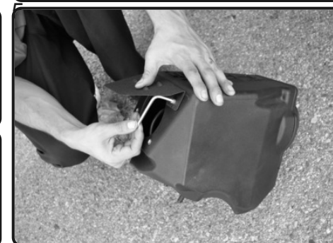
11. Use an allen wrench and remove the Air Box Shield Air Director from the Injen air box. This shield will no longer be used. The snorkel will now be installed.
