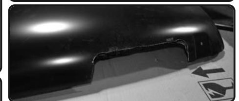
8. This is what it will look like once you have make your cuts with the air saw
