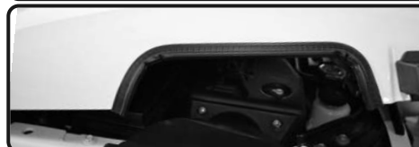
10. Place the 16" vinyl trim onto the edge of the cut out. Re-install your hood and the snorkel is ready for installation
